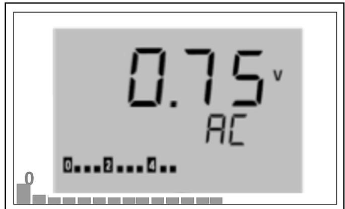
Figure 9. AC voltage display
