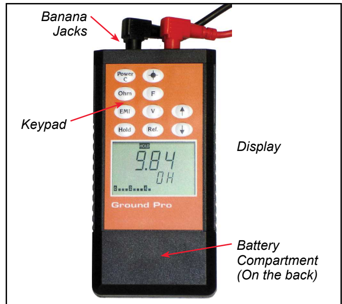
Figure 2. Ground Pro Meter features and components
