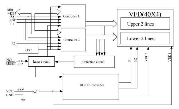
Upper 2 lines are controlled by Controller 1 with E1 signal, and Lower 2 lines are controlled by Controller 2 with E2 signal.
