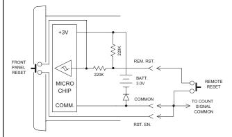
Connecting a wire from the "RST. EN." (Reset Enable) Input terminal to Common will enable the front panel Reset button. When Remote Reset is required, a wire is connected from the "REM. RST." input terminal to Common. Pulling this input low causes the counter to reset. The "REM. RST." can be pulled low by either a mechanical switch or solid-state transistor switch. Switch load and leakage are the same as for "L.S. CNT." Input above.
