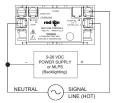
Optional backlight versions of the CUB4 require an external 9-28 VDC power supply. The external supply is connected between the V+ and Common terminals as shown in the drawing.
