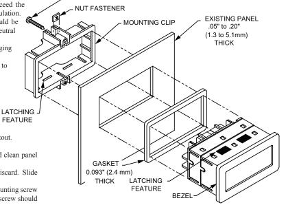
Visually inspect the gasket for proper seal. The gasket should be compressed approximately 75 to 80% of its original thickness. (Recommended torque is 28 to 36 in-oz.)
