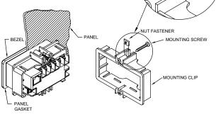
The panel latch should be engaged in the farthest forward slot possible. To achieve a proper seal, tighten the latch screws evenly until the unit is snug in the panel (Torque to approx. 28 to 36 in-oz [0.202 to 0.26 N-m]). Do not overtighten the screws.
