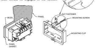
forward slot possible. To achieve a proper seal, tighten the latch screws evenly until the unit is snug in the panel (Torque to approx. 28 to 36 in-oz [0.202 to 0.26 N-m]). Do not over-tighten the screws.
