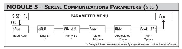
Module 5 is the programming module for the Serial Communications Parameters. The only parameters of concern when utilizing the CUB5USB programming option card to communicate with Crimson 2 programming software is the Baud Rate and Meter Address. The Parameters are only accessible when an optional CUB5USB, RS232 or RS485 serial communications card is installed in the meter.
