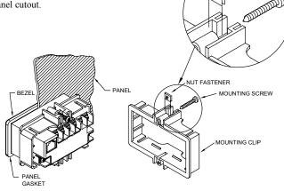
While holding the unit in place, push the panel latch over the rear of the unit so that the tabs of the panel latch engage in the slots on the case. The panel latch should be engaged in the farthest forward slot possible. To achieve a proper seal, tighten the latch screws evenly until the unit is snug in the panel (Torque to approx. 28 to 36 in-oz [0.202 to 0.26 N-m]). Do not over-tighten the screws.
