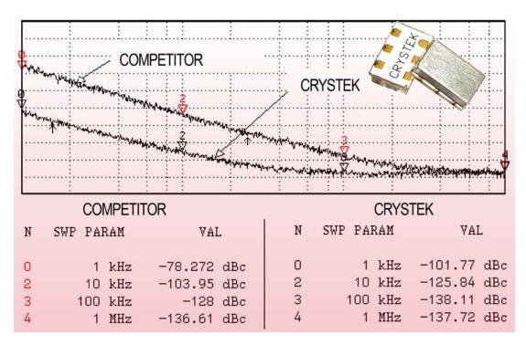
Model CVS575 is a SAW(surface acoustic wave) based Voltage Controlled Oscillator (VCSO) designed for High Performance PLLs. It is an ideal choice for Telecommunication applications needing to meet Low Jitter generation requirements.
