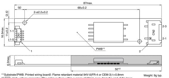
\*'Substrate (PWB: Printed wiring board): Flame retardant material 94V-0(FR-4 or CEM-3) t=0.8mm
