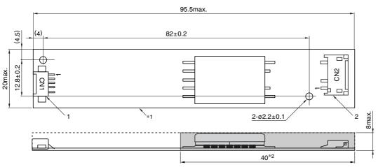
\*1 Substrate (PWB: Printed wiring board): Flame retardant material UL94V-0 (FR-4 or CEM-3) t=1mm
