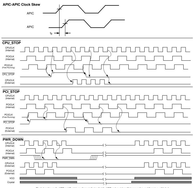
Shaded section on the VCO and Crystal waveforms indicates that the VCO and crystal oscillator are active, and there is a valid clock.
