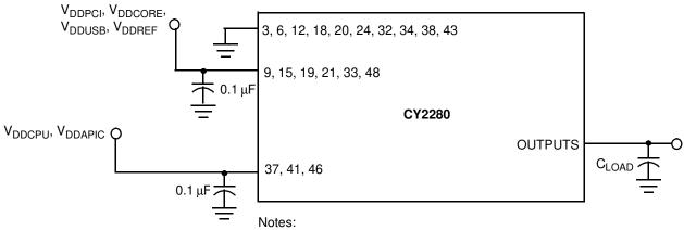
Each supply pin must have an individual decoupling capacitor. All capacitors must be placed as close to the pins as is possible.
