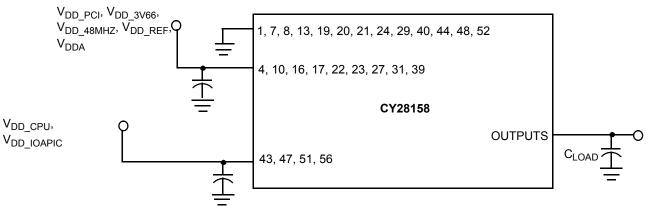
Note: Each supply  $\overline{pin}$  must have an individual decoupling capacitor on test circuit at 0.1  $\mu$ F. Note: All capacitors must be placed as close to the pins as is physically possible.
