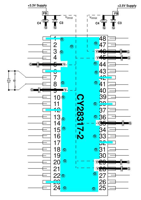
$\label{eq:FB} \begin{array}{l} \mbox{FB = Dale ILB1206 - 300 (300\Omega @ 100 MHz) or TDK ACB2012L-120} \\ \mbox{Ceramic Caps } C3 = 10\mbox{--}22 \ \ \mu\mbox{F} \ \ C4 = 0.005 \ \ \mu\mbox{F} \ \ C6 = 0.01 \ \ \mu\mbox{F} \end{array}$
