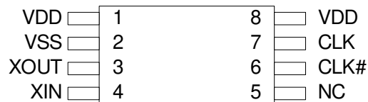
Figure 1. Pin Diagram - 8-Pin TSSOP
