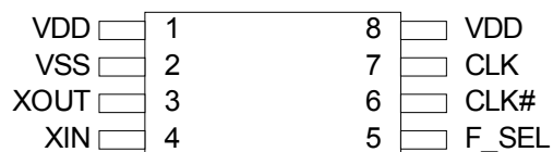
Figure 1. 8-pin TSSOP pinout
