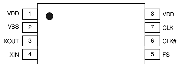
Figure 1. Pin Diagram – 8 Pin TSSOP
