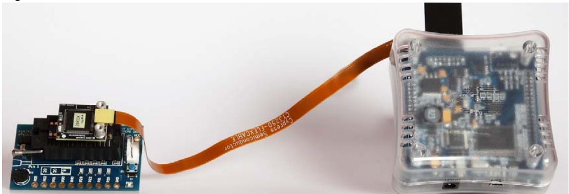
Figure 3-10. Flex Pod Connected to ICE-Cube Pod
