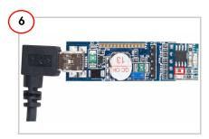
LED D1 of CY3240 USB-I2C Bridge and LEDs D3 and D2 of demo board light up.
