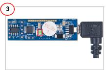
Connect the USB A to Mini B cable and the bridge to the PC. LED D2 (green) lights up.
