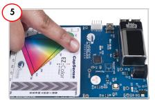
To put the board to "sleep" while powered, press and hold the circular emblem to the left of the CapSense logo.
