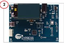
Insert the 9-V battery into the battery holder. Press firmly in place.
