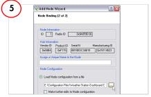
Click 'Load Node configuration from a file' and select Weather\_Station\_Dashboard\_ Configuration.xml from the CD.
