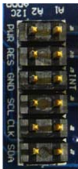
Figure 3-8. Six Jumpers Available on Board
