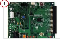
Remove CY3280-20x66 Universal CapSense Controller Board from package. Connect the CY3280-SLM board (to be purchased separately) to the P2 connector.
