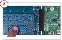
Touch the CapSense button or slider. The respective LEDs lights up.
