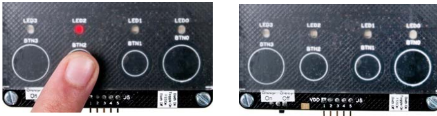
Figure 3-13. Kit with LED On Time Feature Disabled
