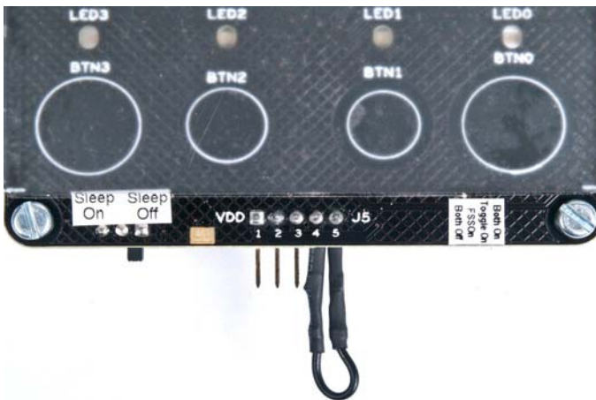
Figure 3-22. BTN1 Sensor Shorted to Ground
