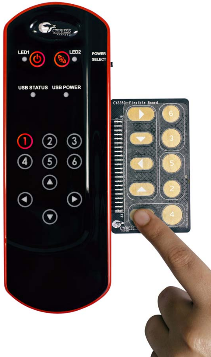
Figure 3-3. Demonstration of SmartSense Auto-Tuning with Flex-PCB
