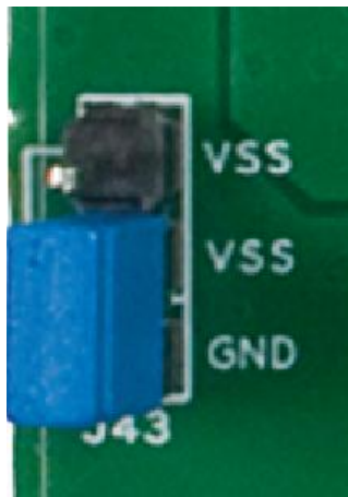
Figure 4-8. Jumper Setting for Ground Reference
