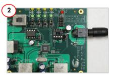
Plug the wall mounted power supply into an AC power receptacle providing power in the range 100 V to 240 V, 50 Hz or 60 Hz. Connect the power supply plug to the hub's 'DC Supply' jack.
