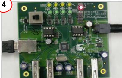
Connect a USB device to any of the four downstream ports. Use jumpers J7 to J10 in position 2-3 to enable the corresponding port status LEDs. The red LED glowing indicates that the hub is not in Suspend mode. The green LED glowing indicates that the respective downstream port is enabled.
