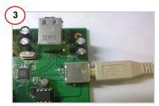
To connect to the PC, plug the USB A to B cable into the hub's upstream connector. Plug the other end of the cable into one of the PC's host controller ports.
