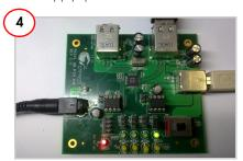
Connect a USB device to any of the four downstream ports. Use jumpers J7 to J10 (port status) in position 2 or 3 to enable the port LEDs. The green LED indicates that the port is enabled.
