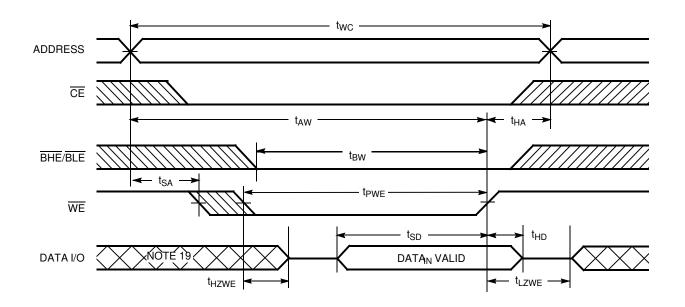
Write Cycle No. 4 (BHE/BLE Controlled, OE LOW)<sup>[18]</sup>
