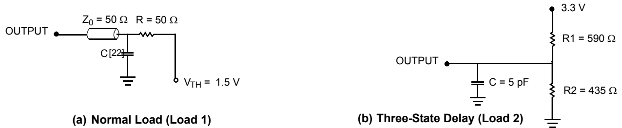
Figure 3. AC Test Loads and Waveforms
