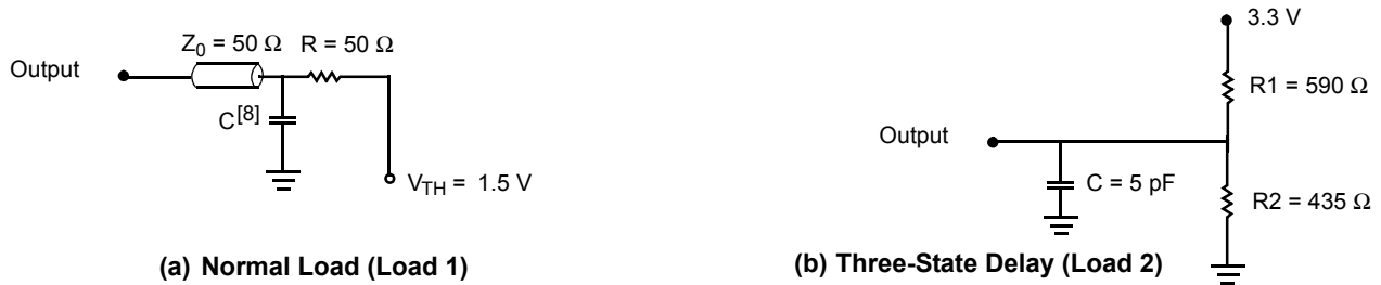
Figure 3. AC Test Load and Waveforms
