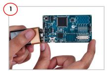
Connect the 9-V battery to the board.
