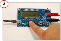
Press the source button to toggle between voltage inputs (Thermocouple and test leads).
