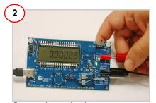
Connect the test leads. CAUTION The input range is limited to -30V DC to +30V DC DO NOT use AC voltage.
