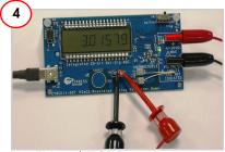
Use TP1 and TP2 test points to measure kit power source.
