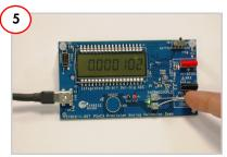
Touch thermocouple and monitor voltage displayed on LCD.
