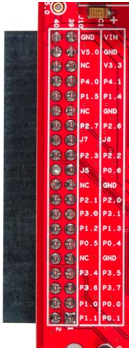
Figure 4-7. Pinout Selections of 40-Pin Header
