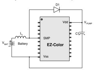
Figure 6. Basic Switch Mode Pump Circuit
