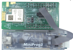
Fig 3: Programming/Debugging with MiniProg3
