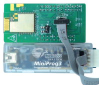
Fig 3: Programming/Debugging with MiniProg3
