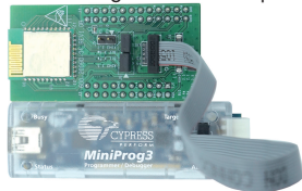
Fig 3: Programming/Debugging with MiniProg3
