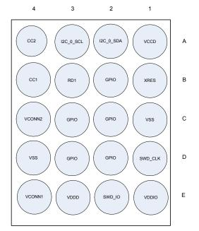
Figure 3. 20-ball WLCSP EZ-PD CCG2 Ball Map (Bottom (Balls Up) View)
