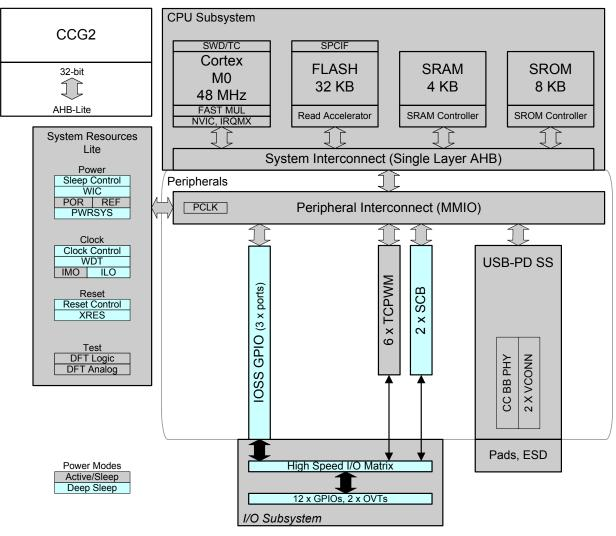
Figure 1. EZ-PD CCG2 Block Diagram
