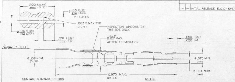
A. CONTACTS: INNER-COPPER ALLOY, GOLD PLATED PER MIL-G-45204 OVER NICKEL UNDERPLATE
