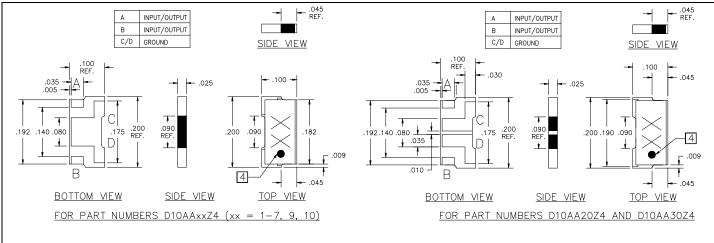
THE D10AAxxZ4 SERIES OF ATTENUATORS ARE SYMMETRICAL UNLESS OTHERWISE SPECIFIED ALL DIMENSIONS ARE IN INCHES
