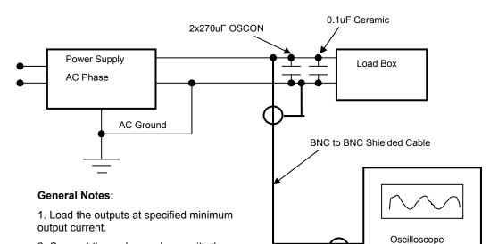
2. Connect the probe as shown with the input tip and ground as short as possible.
