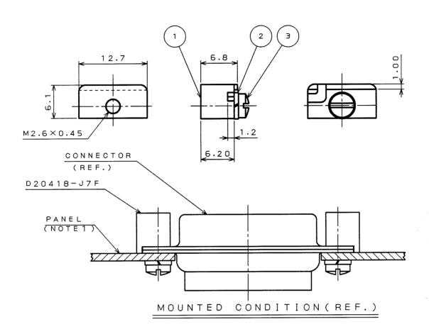
NOTE1.APPLICABLE PANEL THICKNESS IS MORE 1.2 LESS THAN 1.7. LENGTH OF ATTACHED SCREW IS 5.5[mm]
