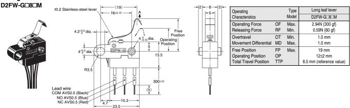
Note1. Unless otherwise specified, a tolerance of ±0.4 mm applies to all dimensions. Note2. The operating characteristics are for operation in the A direction (  $\clubsuit$  ).
