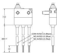
UL approved wires (AWG24, UL1007) are used for UL/CSA standard approved items.
