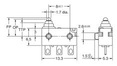
Note. The reference positions used for Free Position (FP), Operating Position (OP), and Total Travel Position (TTP) values are as shown above for each type of mounting.
