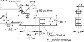
D2MV-1L22-1C3 Model Operating D2MV-01L22-1C3 characteristics Operating Force OF Max 0.49N {50 gf} RF Min. Releasing Force 0.04N {4 gf} (reference value) Pretravel PT Max. 1.7 mm Overtravel OT Min. 1.0 mm Movement Differential MD Max 0.4 mm Operating Position OP 20.7±0.6 mm
