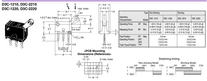
Note 1. Unless otherwise specified, a tolerance of ±0.4 mm applies to all dimensions.
