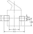
Note 1. Unless otherwise specified, a tolerance of  $\pm 0.15$  mm applies to all dimensions.
