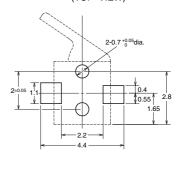
Note 1. Unless otherwise specified, a tolerance of  $\pm 0.15 \ \text{mm}$  applies to all dimensions.
