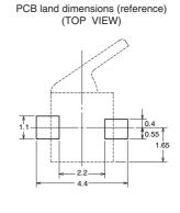
Note 1. Unless otherwise specified, a tolerance of  $\pm 0.15$  mm applies to all dimensions.
