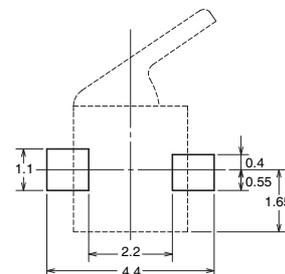
Note 1. Unless otherwise specified, a tolerance of  $\pm 0.15$  mm applies to all dimensions.
