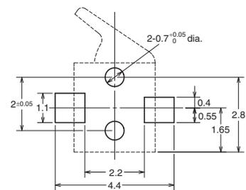
Note 1. Unless otherwise specified, a tolerance of  $\pm 0.15$  mm applies to all dimensions.
