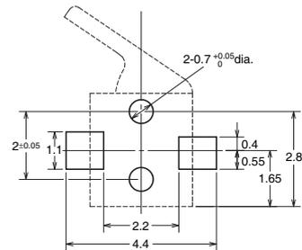
Note 1. Unless otherwise specified, a tolerance of  $\pm 0.15$  mm applies to all dimensions.
