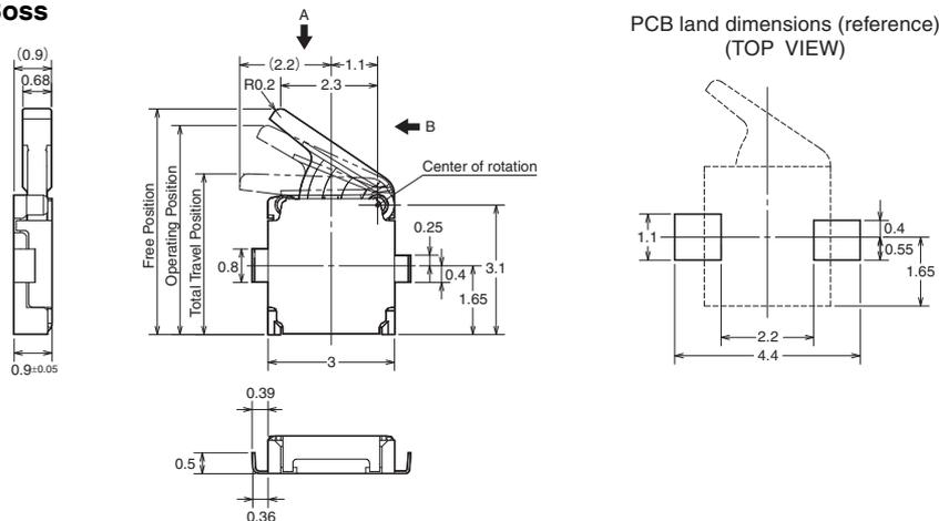
Note 1. Unless otherwise specified, a tolerance of ±0.15 mm applies to all dimensions.
